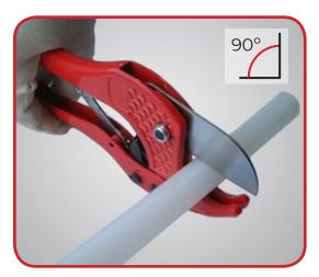
**1.** Cut the pipe as clean and perpendicular as possible to its axis.
