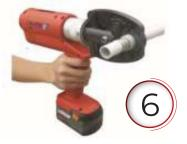
Press with U or TH jaws. If TH jaws are used, the side of the jaw must be placed on the plastic ring.
