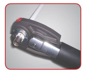
**3.** Place the side of the jaw beside the plastic ring and press with U, RF or RFz jaw. The plastic ring should not be pressed.
