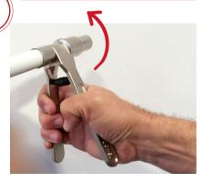
Insert the fitting completely. The pipe must be seen through the check holes of the stainless steel sleeve. The end of the stainless steel sleeve must reach the plastic ring (black or white). Don't leave more than 1,5 mm between the end of the stainless steel sleeve and the plastic ring.
