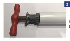
The pipe must be well cut, perpendicularly to its axis. Then, use the reamer to chamfer the pipe.
