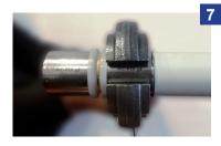
Press with U type jaws or rings. Place the side of the jaw beside the plastic ring and press. The plastic ring should not be pressed.
