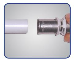
**3.** Insert the fitting into the pipe. The pipe must be seen through the check holes of the sleeve.
