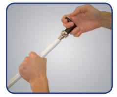
2. It is necessary to calibrate and chamfer the pipe inside in order not to damage the O-Rings of the fittings. The AC-FIX chamfering tool chamfers and calibrates the pipe.
