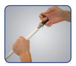
2. It is necessary to calibrate and chamfer the pipe inside in order not to damage the O-Rings of the fittings. The AC-FIX chamfering tool chamfers and calibrates the pipe.
