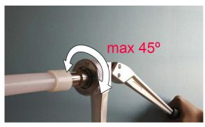
The maximum number of expansions, which must not be exceeded, is shown in the table previously mentioned. At low temperatures the pipe will narrow back more slowly, which means that, depending in the pipe size, the necessary number of expansions will be less than usual for the flat part of the jaws to be all the way inside the pipe.
