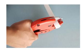
2. Fit the plastic ring into the pipe so that a very small part of it (max. 1mm) is outside the pipe end.
